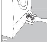
Clean the filter under a running tap, then refit it, screwing it fully in.
